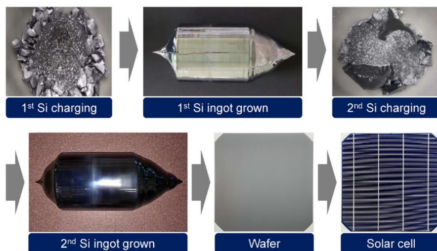
Fig. 5. Overall process flow for preparing c-Si solar cells from recovered silicon waste [37]
