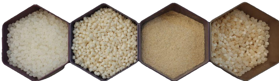
Fig. 1. Materials used for sample preparation: from left: PLA granules, PHB granules, wood fibers and a PLA/PHB (80:20) blend containing 10 \text{ wt}\% wood fibers
