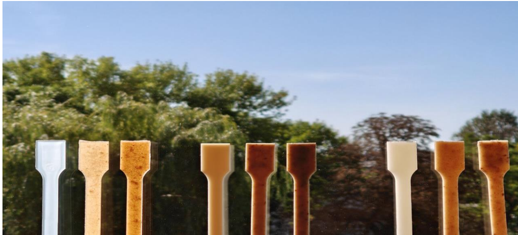
Fig. 2. Photographs of the prepared dumbbell specimens under natural light, categorized by matrix material and filler content. From left to right: PLA, PHB and PLA/PHB (80:20) blend. Within each group, the samples represent 0 wt%, 5 wt% and 10 wt% wood fiber content, respectively
