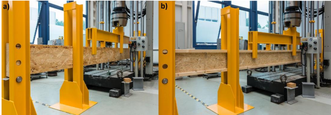
Fig. 1. OSB laminated beam a) and I-beam b) on the test stand
