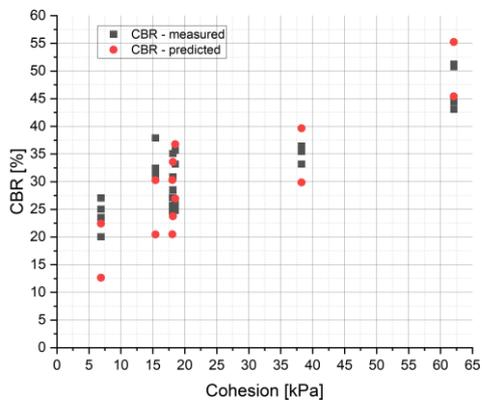
Fig. 15. CBR index values measured and predicted as a function of cohesion
