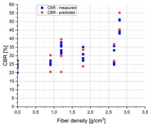
Fig. 13. CBR index values measured and predicted as a function of fiber density
