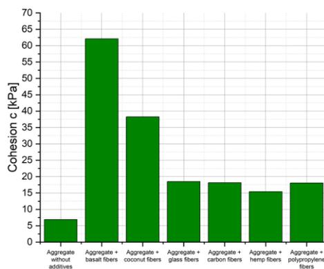
Fig. 10. The cohesion value for samples with fiber additives
