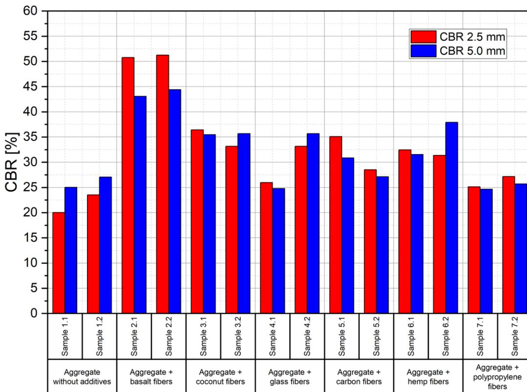
Fig. 9. The CBR index value for samples with fiber additives
