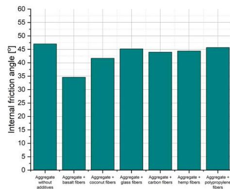
Fig. 11. The internal friction angle for samples with fiber additives
