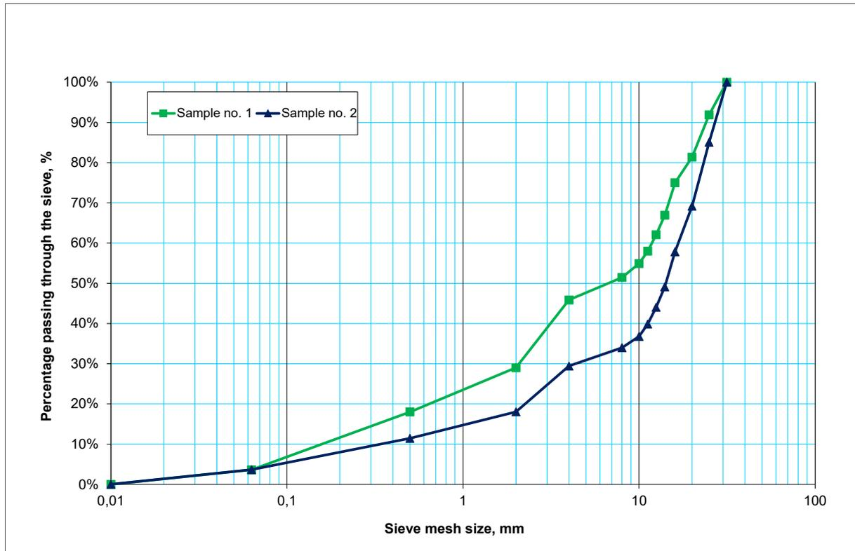
Fig. 7. Grain Size Distribution Curve for Sandstone Aggregate
