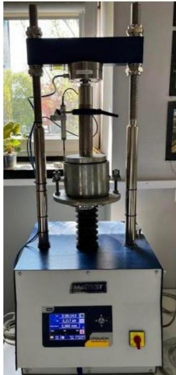
Fig. 8. CBR Testing Press
