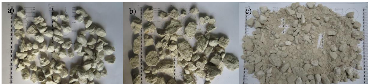
Fig. 3. a, b – characteristic samples differing in aggregate grain shape, c – homogenized aggregate sample for testing in a shear box apparatus
