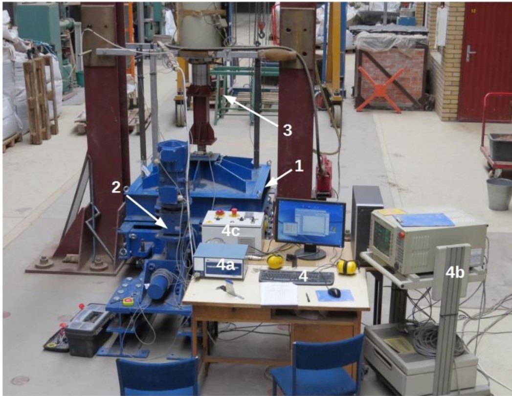
Fig. 5. View of the WABS Test Stand, Testing Position: 1 – Testing chamber, 2 – Test stand drive system, 3 – Schenck press actuator for applying vertical loads, 4 – Test process control station, 4a – GEODATALOG for processing sensor signals, 4b – Schenck press controller, 4c – Test stand drive controller (lead screw) [22]
