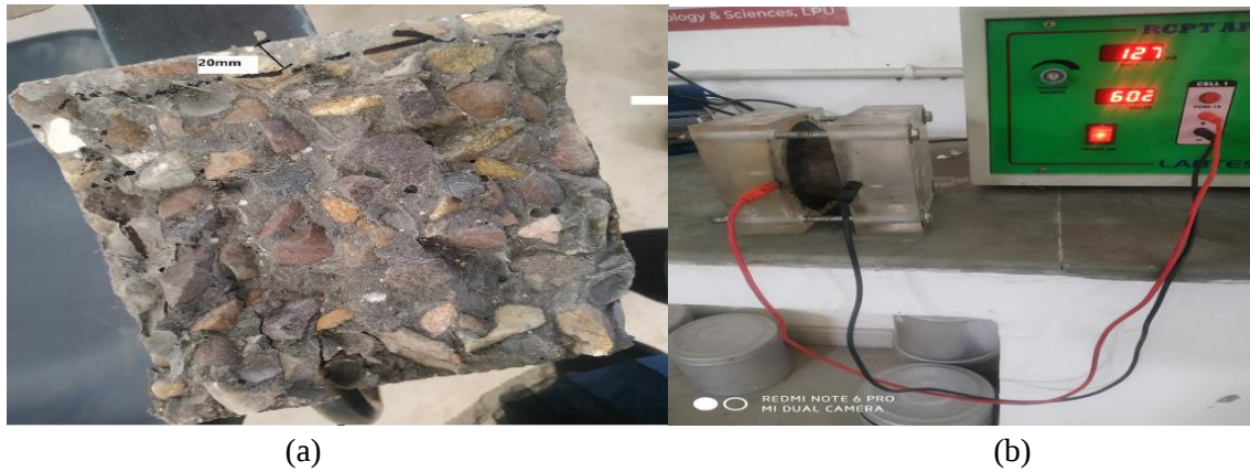
Fig. 5. Durability test (a) Water permeability test (b) RCPT test for developed SCGPC
