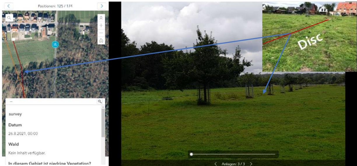
Fig. 8. Detailed view of the application of mobile GIS to map the discontinuities in Grafenwald: Orange line modelled discontinuity (carbon surface), red line - discontinuity on the surface after validation with drone data (left) and in-situ documentation using mobile GIS (right)
