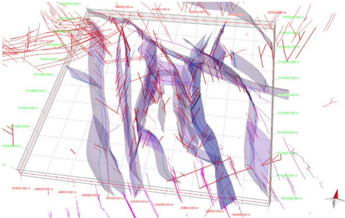
Fig. 4. Oblique view of the modelled faults in the research area
