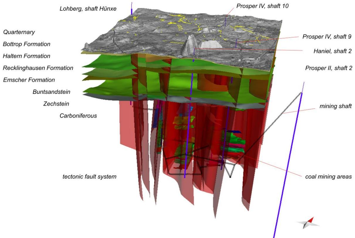
Fig. 5. Oblique view of the overburden model (Exaggeration: 7,5; looking NW) showing the faults (red), the coal mining areas (red, green), the top of the Carboniferous (grey), the upper formations of the overburden (green, orange) and the upper Quaternary below the top surface
