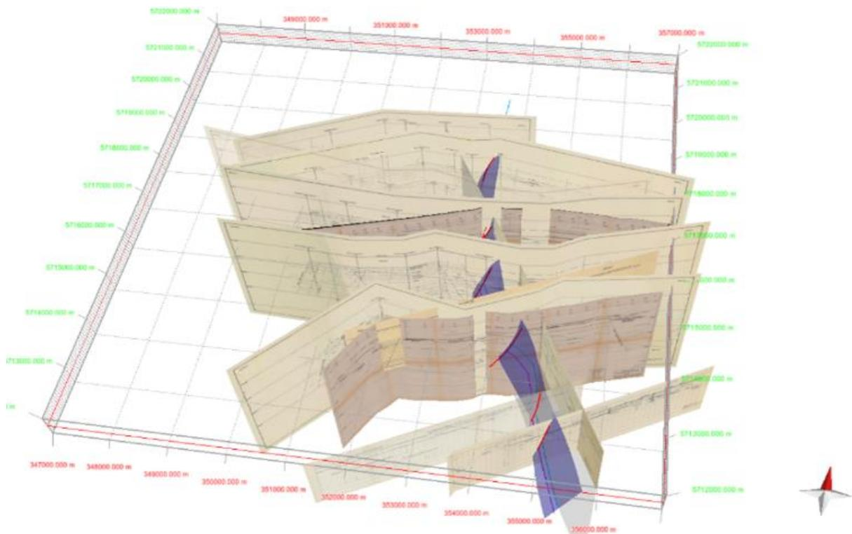
Fig. 3. Oblique view of the modelled Krudenburg fault on the basis of mine survey profiles
