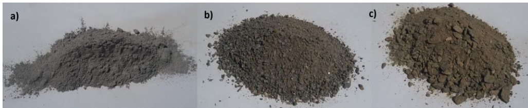
Fig. 1. Recycled amphibolite aggregate: a) dust fraction, b) 0–2 mm fraction, c) 0–5 mm fraction,
