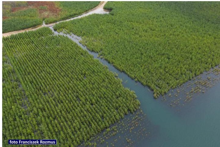
Fig. 2. Aerial view of subsidence lake that developed in the Bolesław post-mining area, August 2024 [33]
