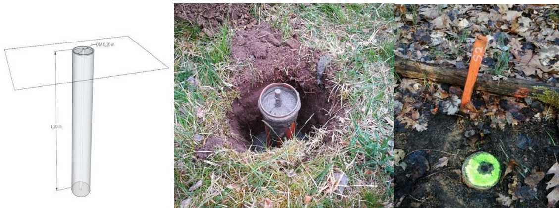
Fig. 3. Design and construction of controlled points
