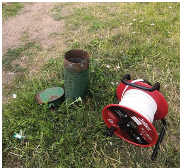
Fig. 4. The top of a measurement point and the measuring device Solinst 107TLC
