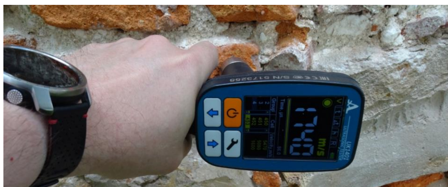
Fig. 23. Test of ultrasonic wave velocity
