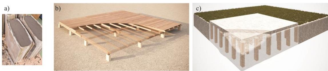
Fig. 4. Proposal 1: Point foundations made of concrete-filled Vestas-type spar caps sections (visualisation - N.Jakubiak, W.Jabłoński): a) ‘prefabricated’ foundation, b) timber house foundation beams supported on point foundations, c) point foundations under a bottom slab
