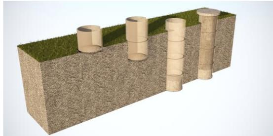
Fig. 5. Proposal 2: Foundation well made of Vestas or LM blade circular sections (visualisation - N.Jakubiak, W.Jabłoński):
