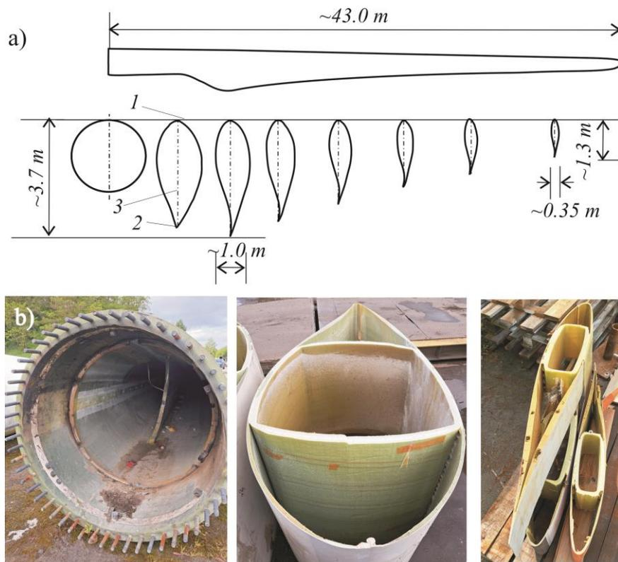
Fig. 3. Cross-sections of wind turbine blades: a) change of cross-section along the blade (figure made on the basis of [34], b) blade cross-sections: circular cross-section near the column, “wide teardrop” transient section, “teardrop” section (photo - Ł. Jabłoński)
