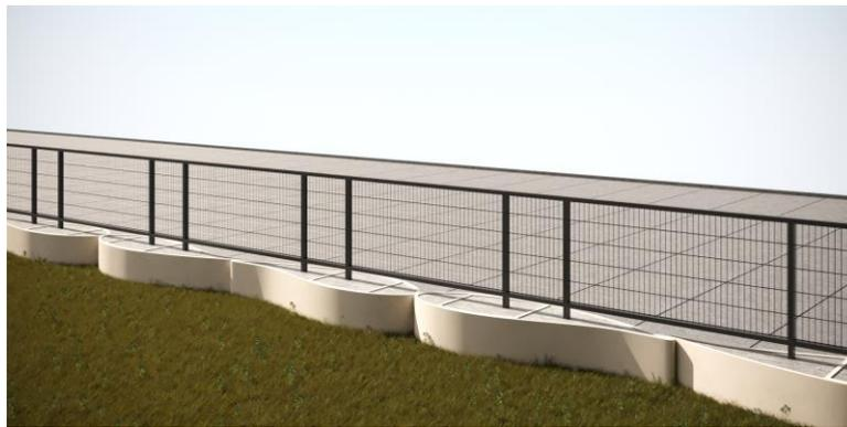
Fig. 6. Proposal 3: Foundations for railings and fences made of LM blades (visualisation - N.Jakubiak, W.Jabłoński)
