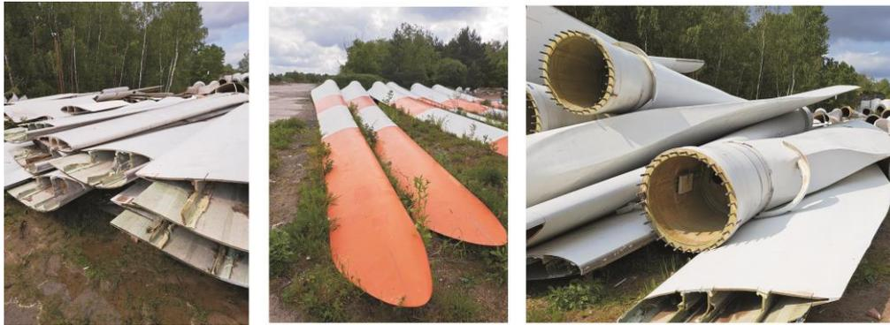
Fig. 1. Wind turbine blades stored in a landfill (photo - Ł. Jabłoński)
