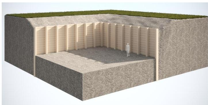
Fig. 9. Proposal 6: Cantilever retaining wall: cantilever beams made of Vestas-type spar caps and plating made of fragments of LM blades (visualisation - N.Jakubiak, W.Jabłoński)
