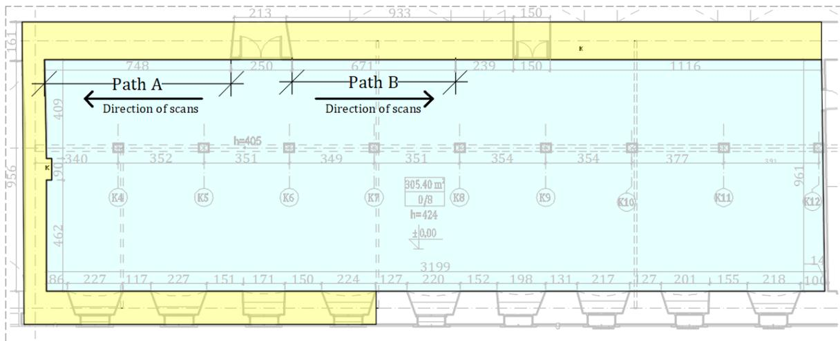
Fig. 3. Excerpt from the ground floor plan indicating the two scan paths analyzed along with the direction of scanning
