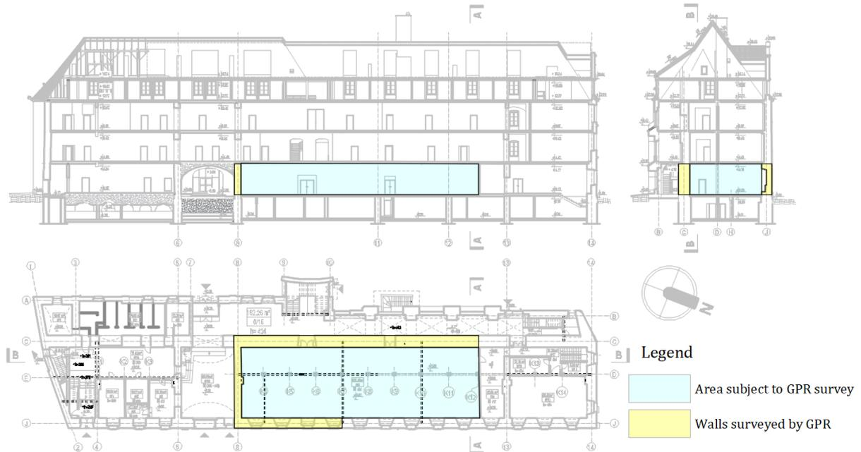
Fig. 2. Situation plan showing the subject of the GPR survey. Elaboration based on [19]
