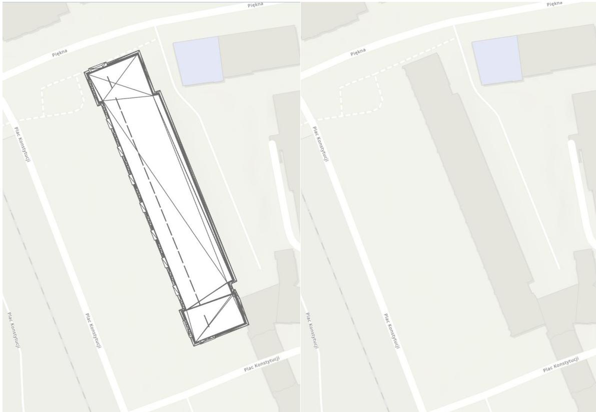
Fig. 5. The building model in 2D view after georeferencing and coordinates (left) and the location of the building against a topographic map from ESRI (right) in ArcGIS Pro. Source: own development
