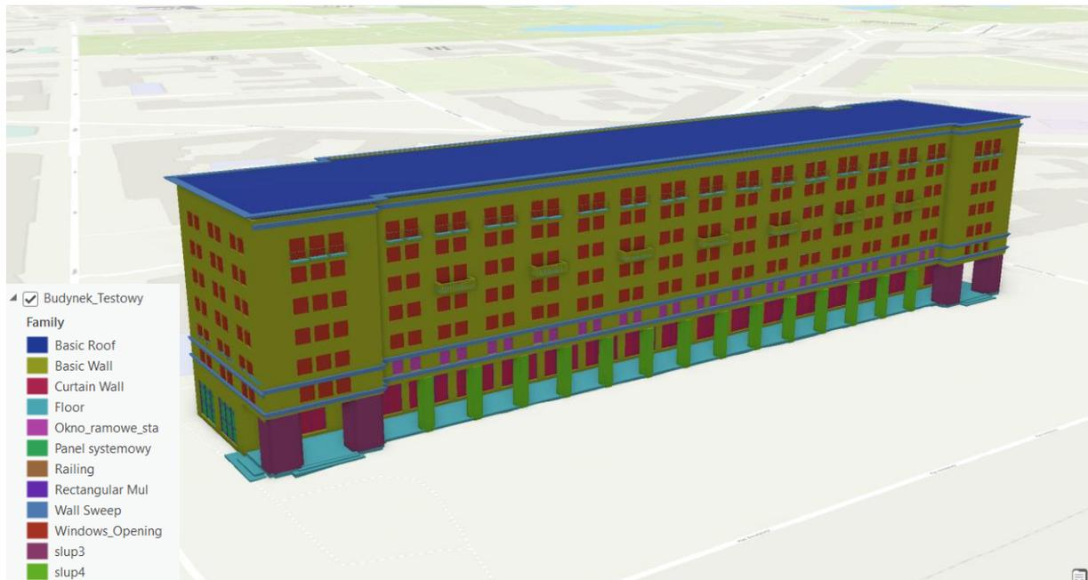
Fig. 10. Color breakdown of the building model based on Revit families. Source: own development
