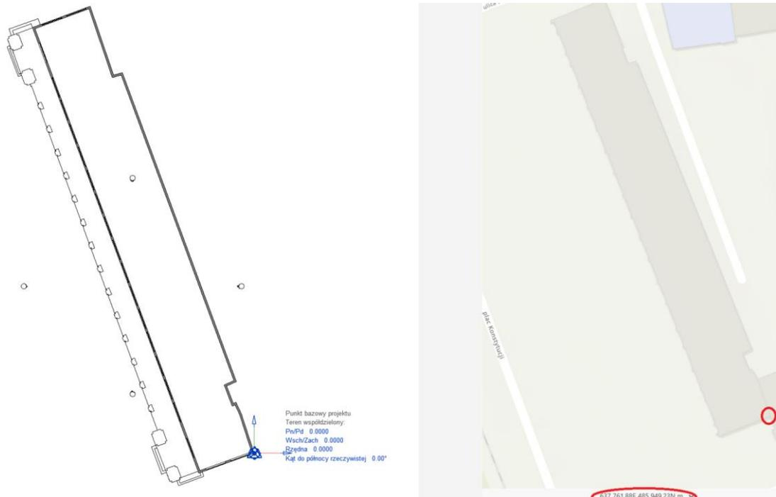
Fig. 3. Setting the base point to a known base point and checking the X and Y coordinates. Source: own development
