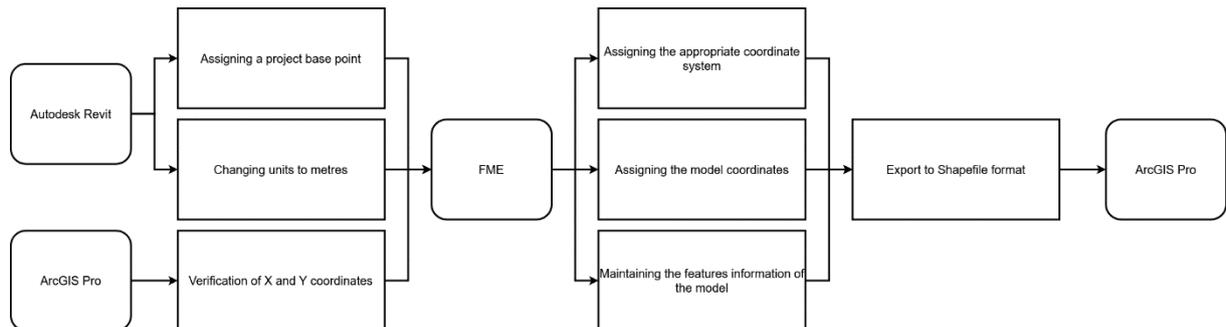
Fig. 2. Flow chart of the procedure process. Source: own development
