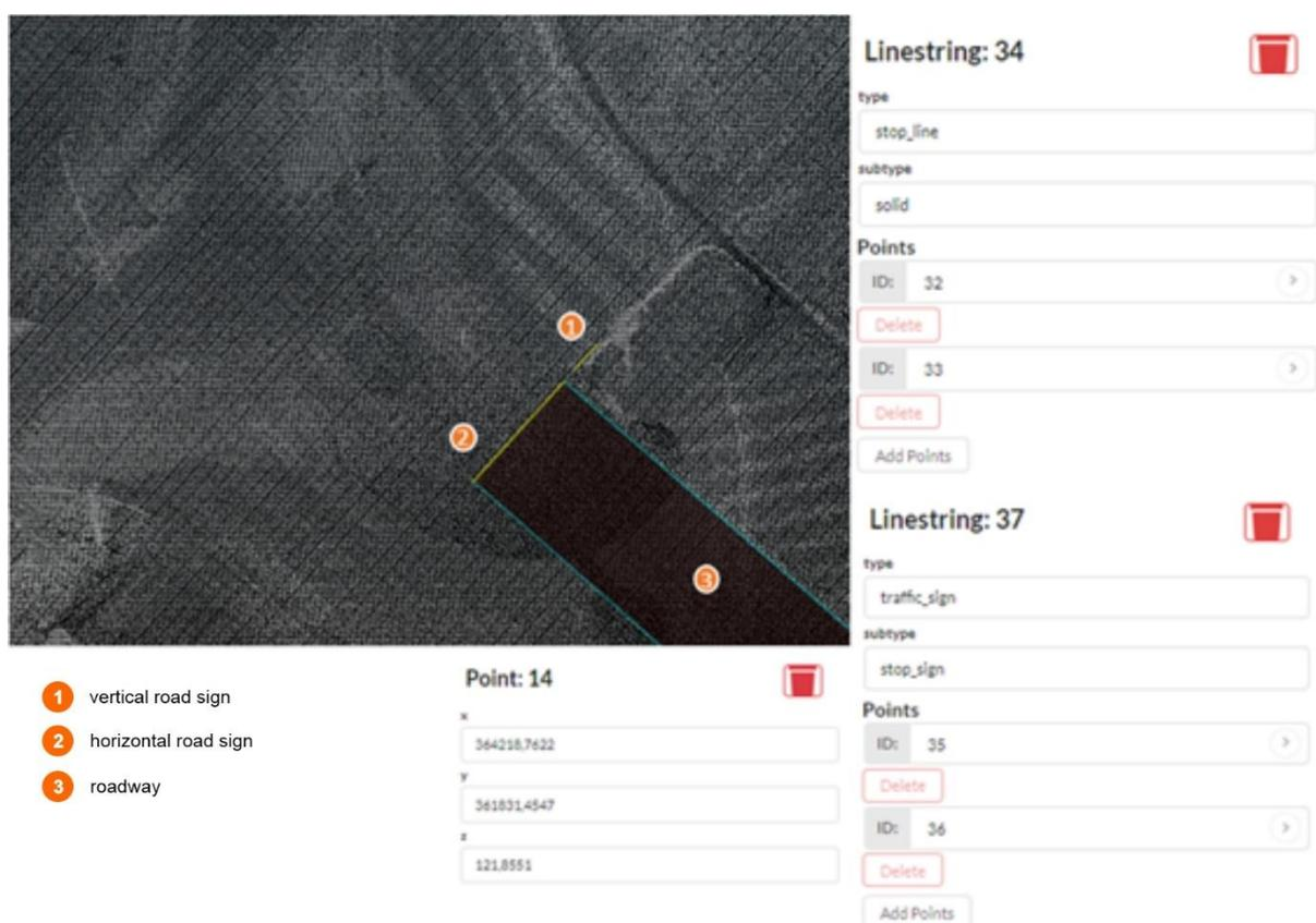
Fig. 10. The vectorization and encoding process of individual horizontal elements
