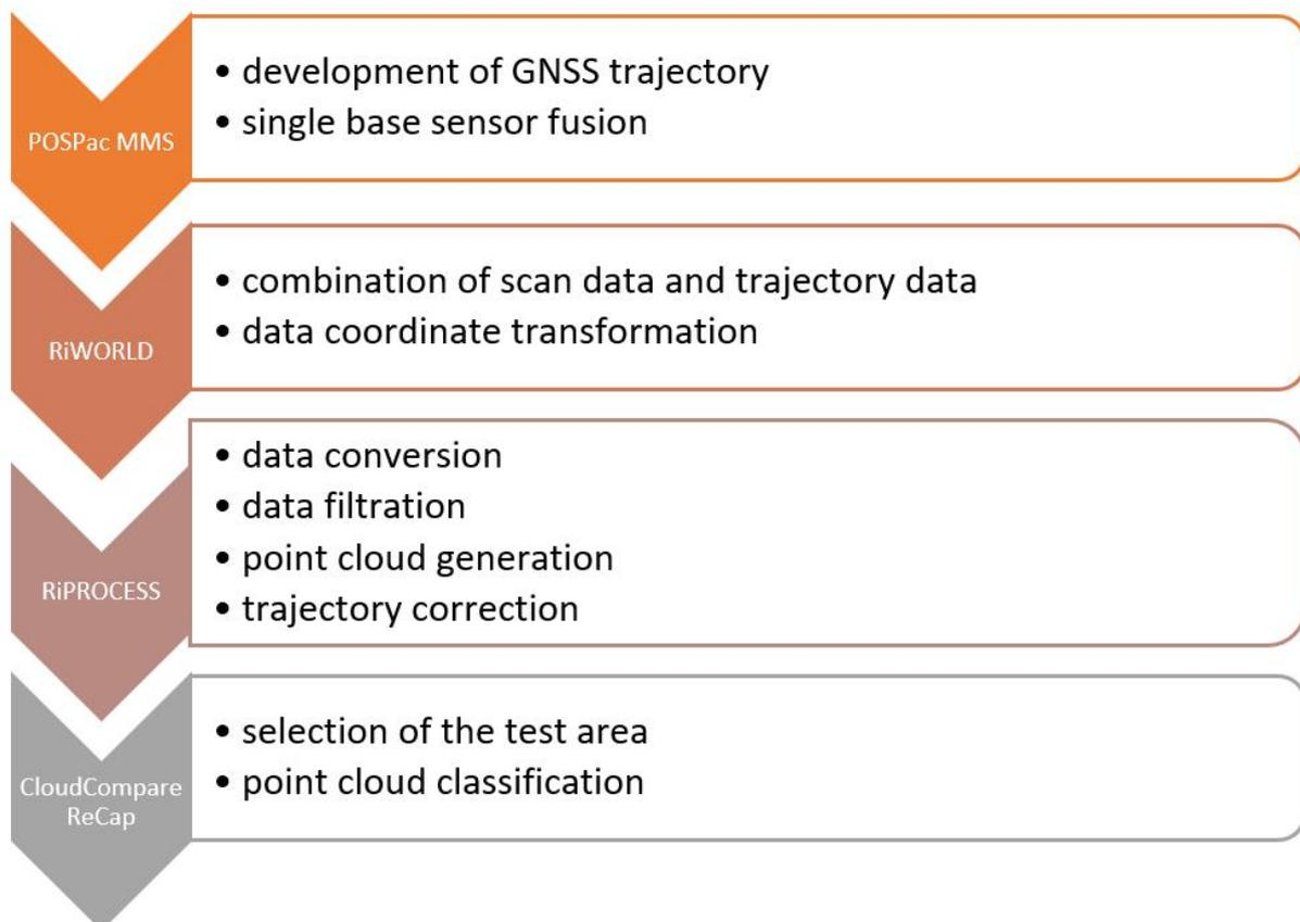
Fig. 4. Schematic diagram of MLS data pro-processing
