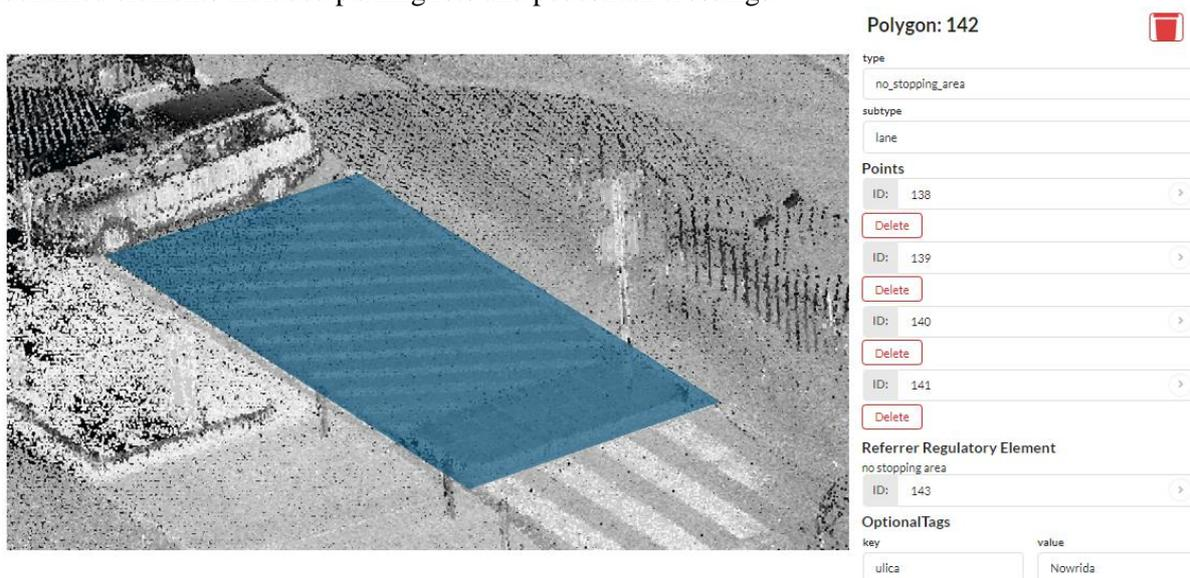
Fig. 12. Visual representation of a fragment of the test area which does not carry the traffic defined in the HD map
