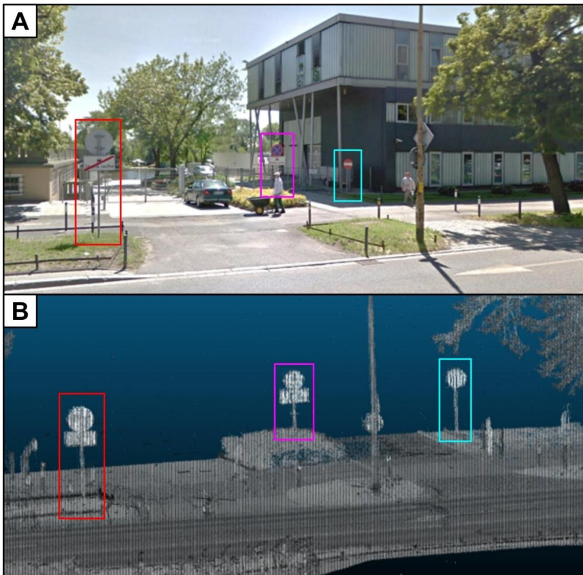
Fig. 9. Identification of road sign types: (A) Google Street View; (B) point cloud
