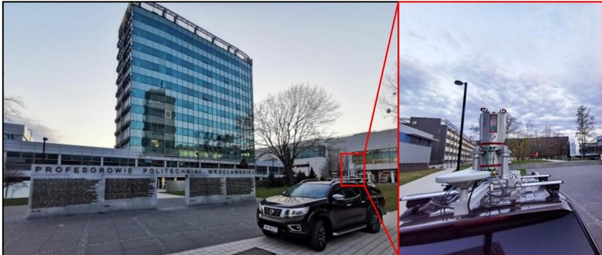
Fig. 2. Riegl VMZ 400i during the data acquisition process in the Professor Alley (main WUST campus)
