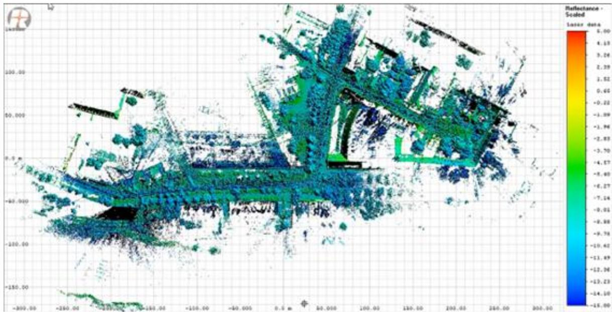
Fig. 5. 2D representation of the point cloud (data records) with the applied trajectory
