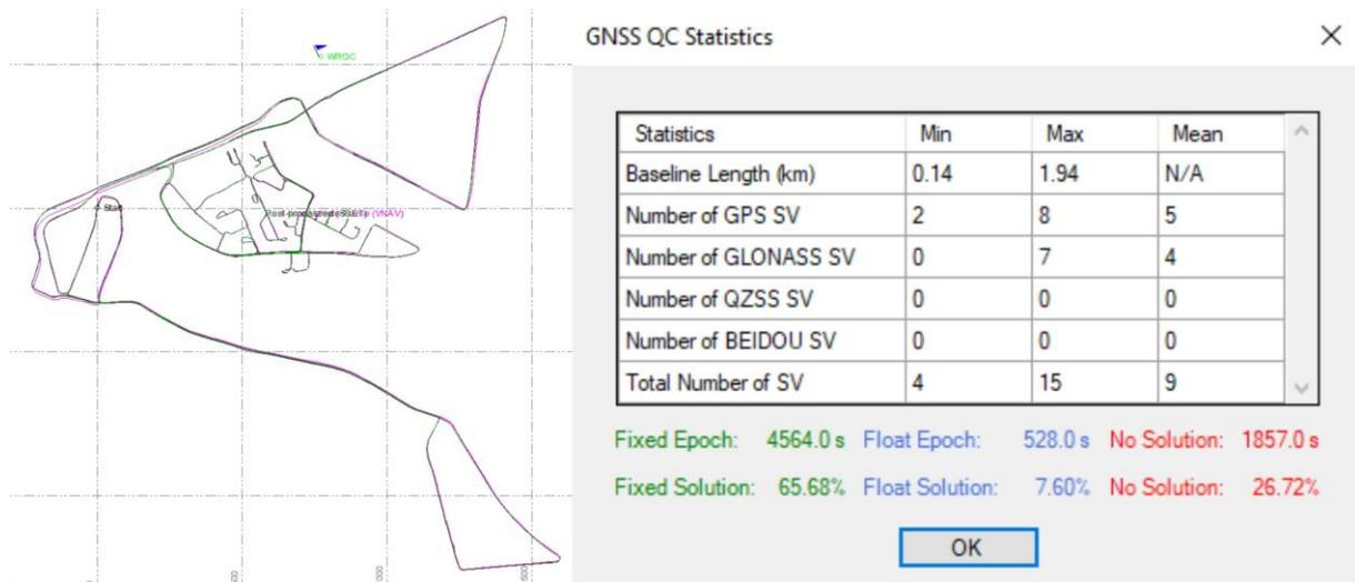
Fig. 3. Results of trajectory processing based on the GNSS WROC base station
