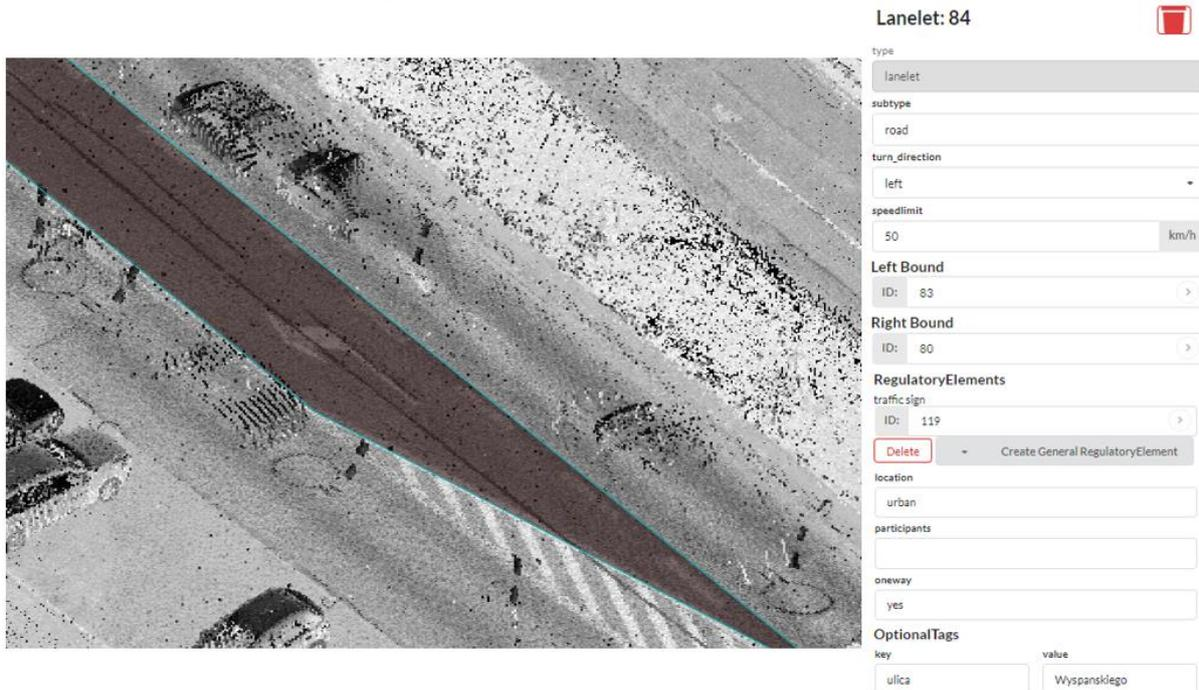
Fig. 11. Visual representation of a road lane vectorized with Vector Map Builder and with defined relations
