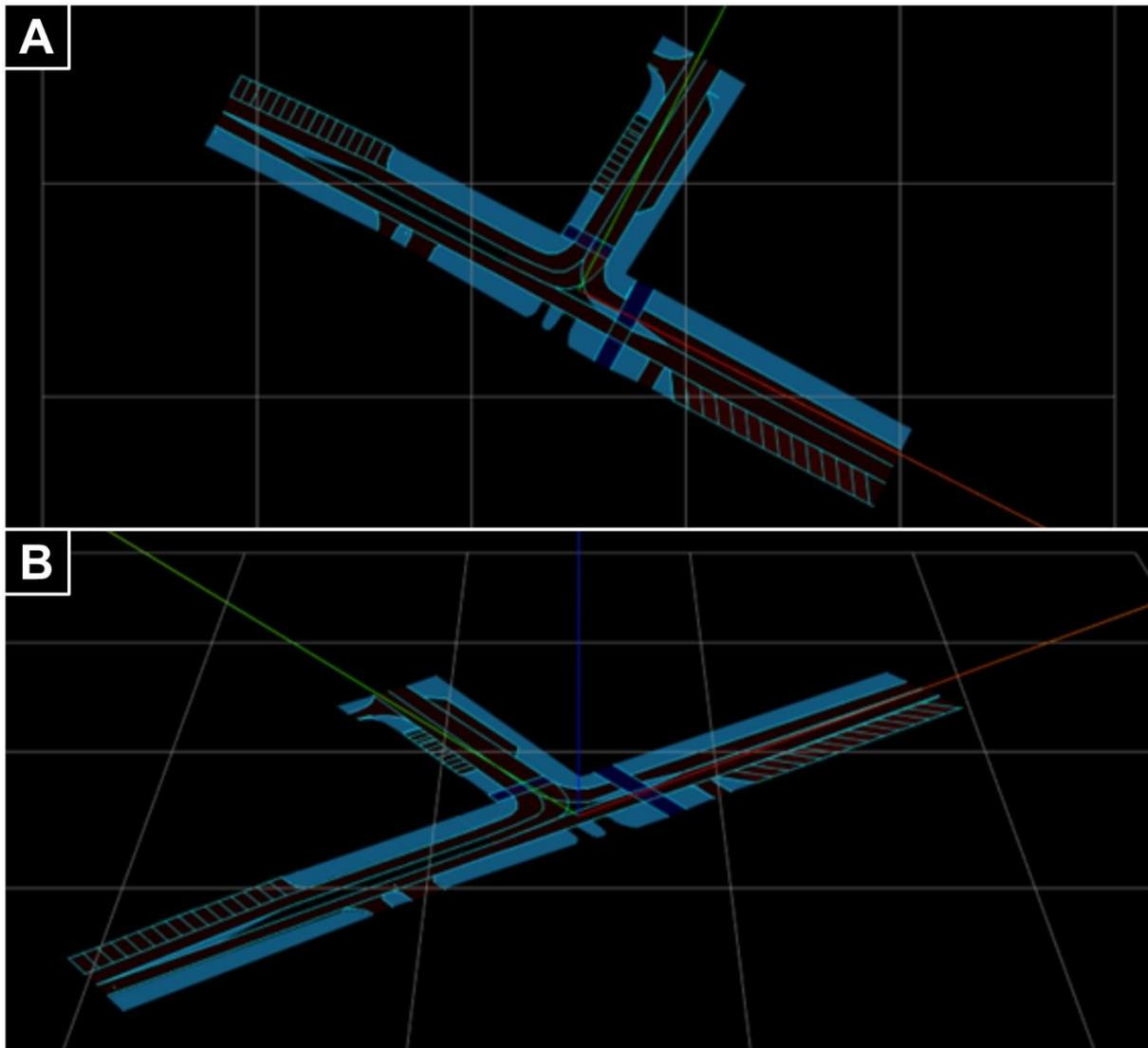
Fig. 13. Visual representation of the final HD map for autonomous vehicles developed for the WUST campus:
