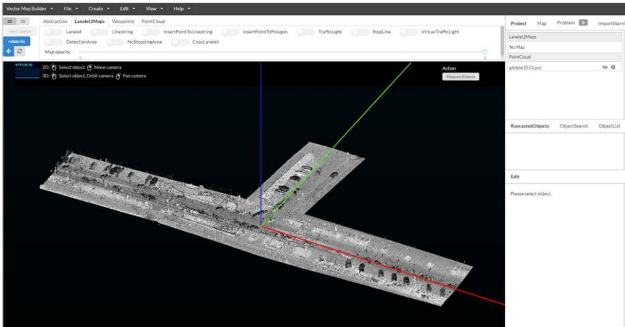
Fig. 8. Input point cloud in the Vector Map Builder environment
