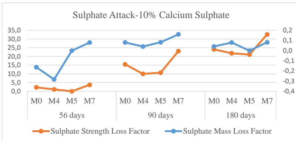
Fig. 10. Variation of Sulphate Mass Loss Factor and Sulphate Strength Loss Factor with 10% Calcium Sulphate solution
