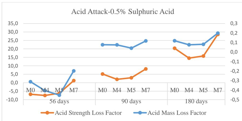
Fig. 7. Variation of Acid Mass Loss Factor and Acid Strength Loss Factor with 0.5% Sulphuric acid
