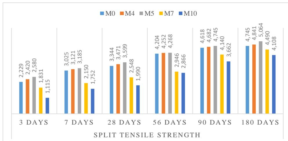
Fig. 5. Split tensile strength variation of the mixes
