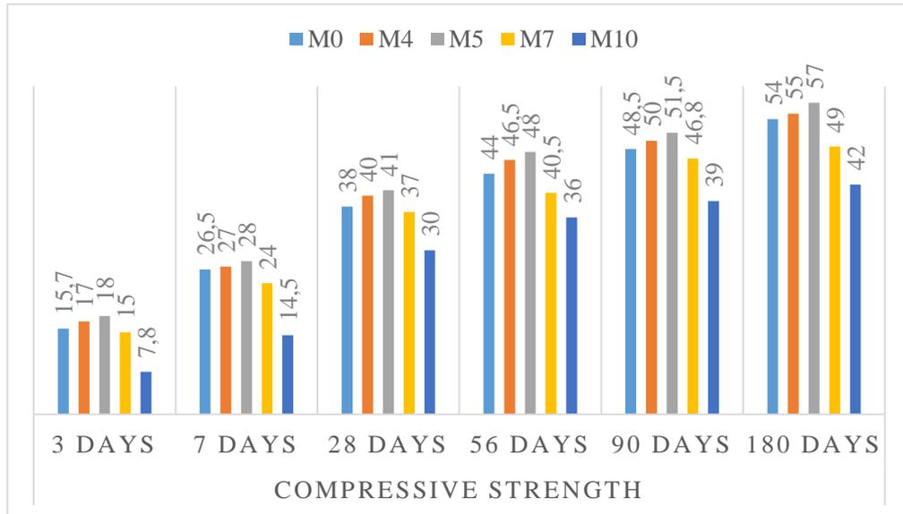
Fig. 4. Compressive strength variation of the mixes
