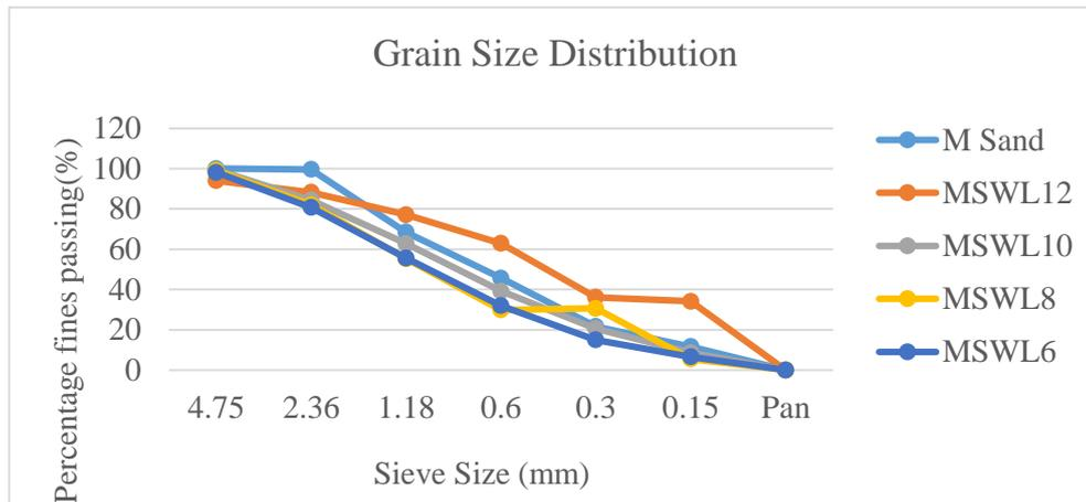
Fig.1. Particle size distribution of M Sand and MSWL Samples
