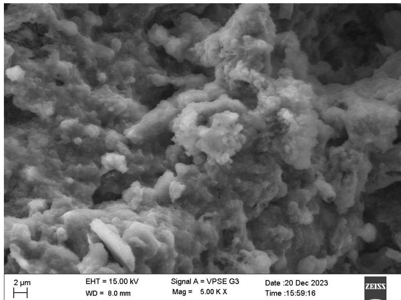
Fig. 4. SEM images of mixes with 5000 magnification of a) Normal concrete b) MSWL concrete
