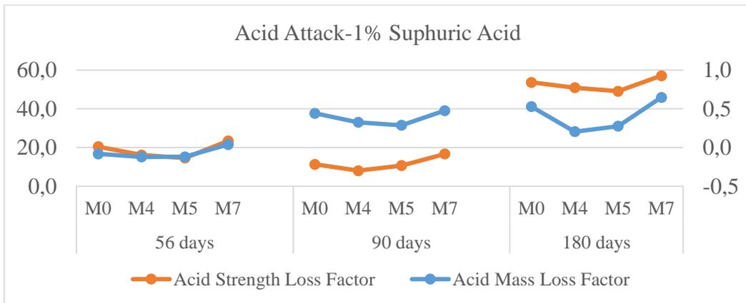
Fig.8. Variation of Acid Mass Loss Factor and Acid Strength Loss Factor with 1% Sulphuric acid
