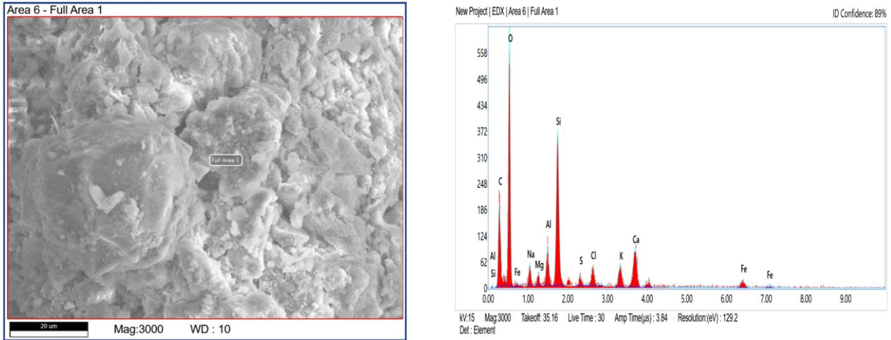
Fig. 3. a) Scanning Electron Microscope (SEM) and b) Energy-Dispersive X-ray microanalysis Test (EDAX) of MSWL 12
