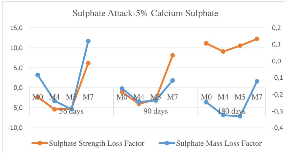
Fig. 9. Variation of Sulphate Mass Loss Factor and Sulphate Strength Loss Factor with 5% Calcium Sulphate solution
