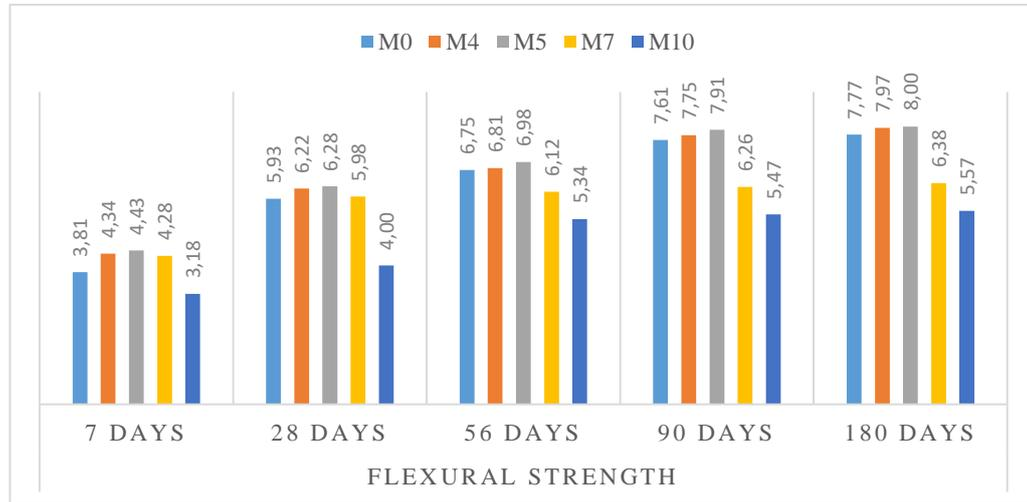
Fig. 6: Flexural strength variation of the mixes
