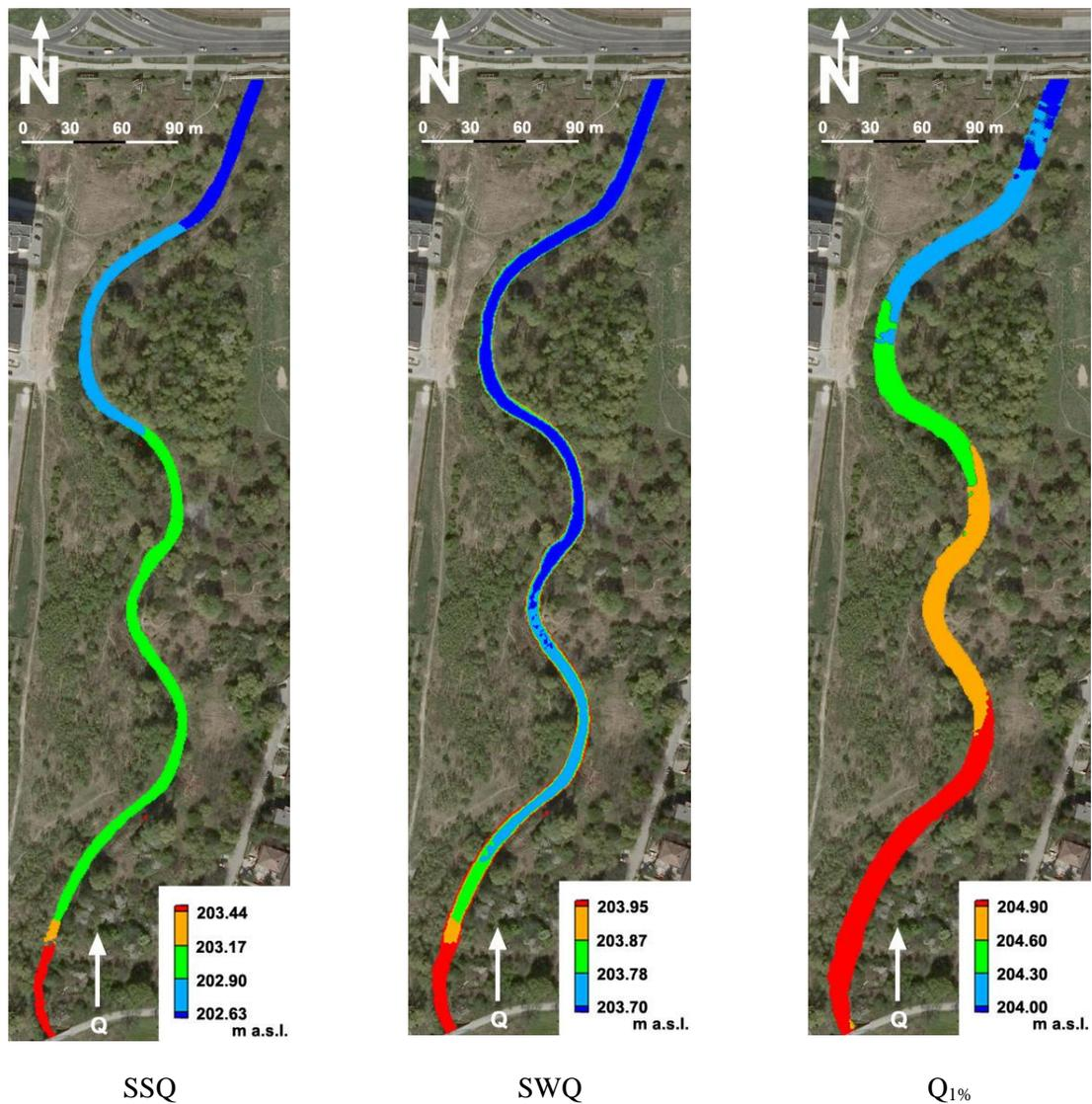
Fig. 6. The surface water table in the watercourse for the multiannual mean low flow (a) and mean annual maximum flows (b)
