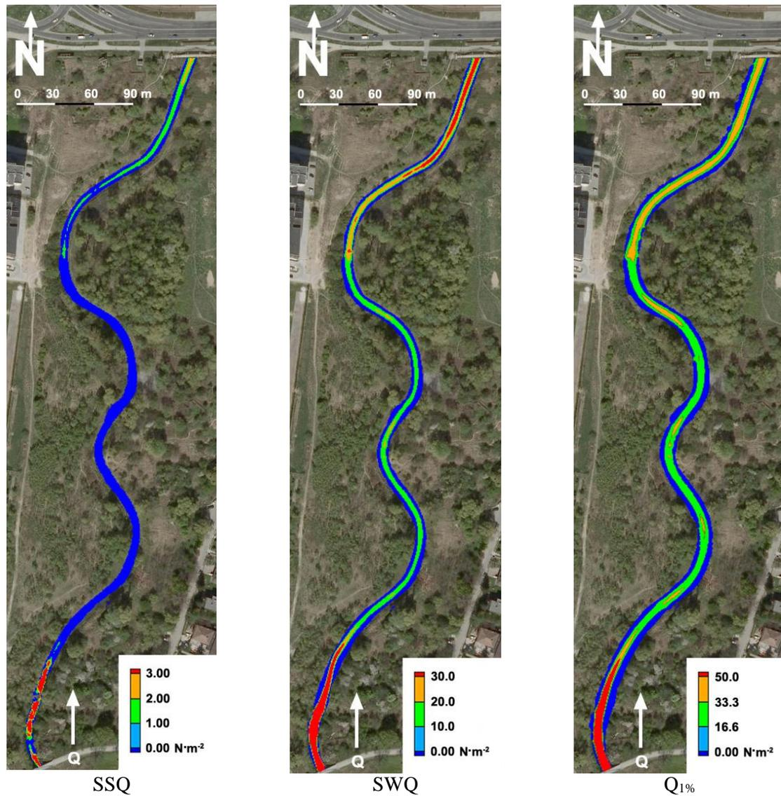
Fig. 4. Shear stress in the watercourse for the multiannual mean low flow (a) and mean annual maximum flow (b)
