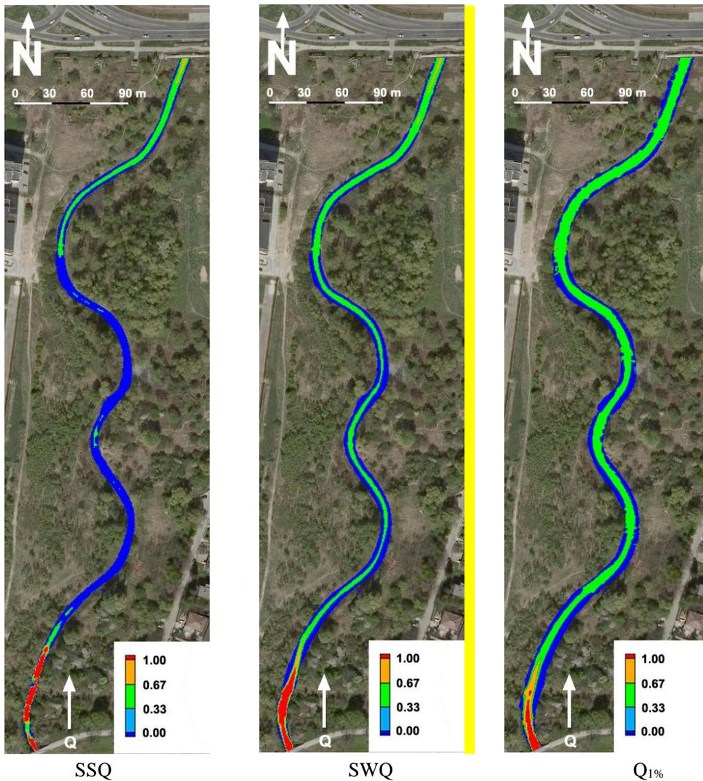
Fig. 5. The Froude number in the watercourse for the multiannual mean low flow (a) and mean annual maximum flows (b)
