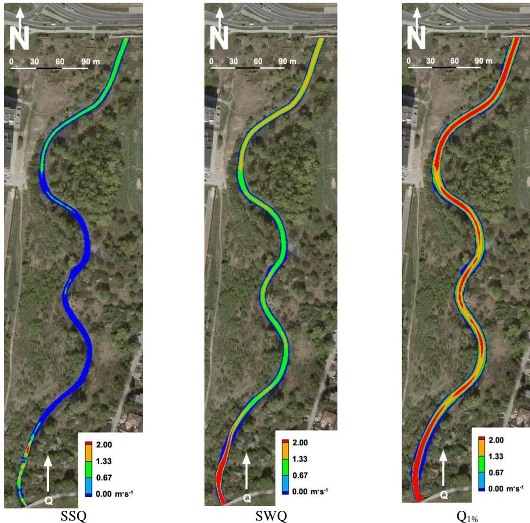
Fig. 2. The velocity in the watercourse for the multiannual mean low flow (a) and mean annual maximum flows (b)
