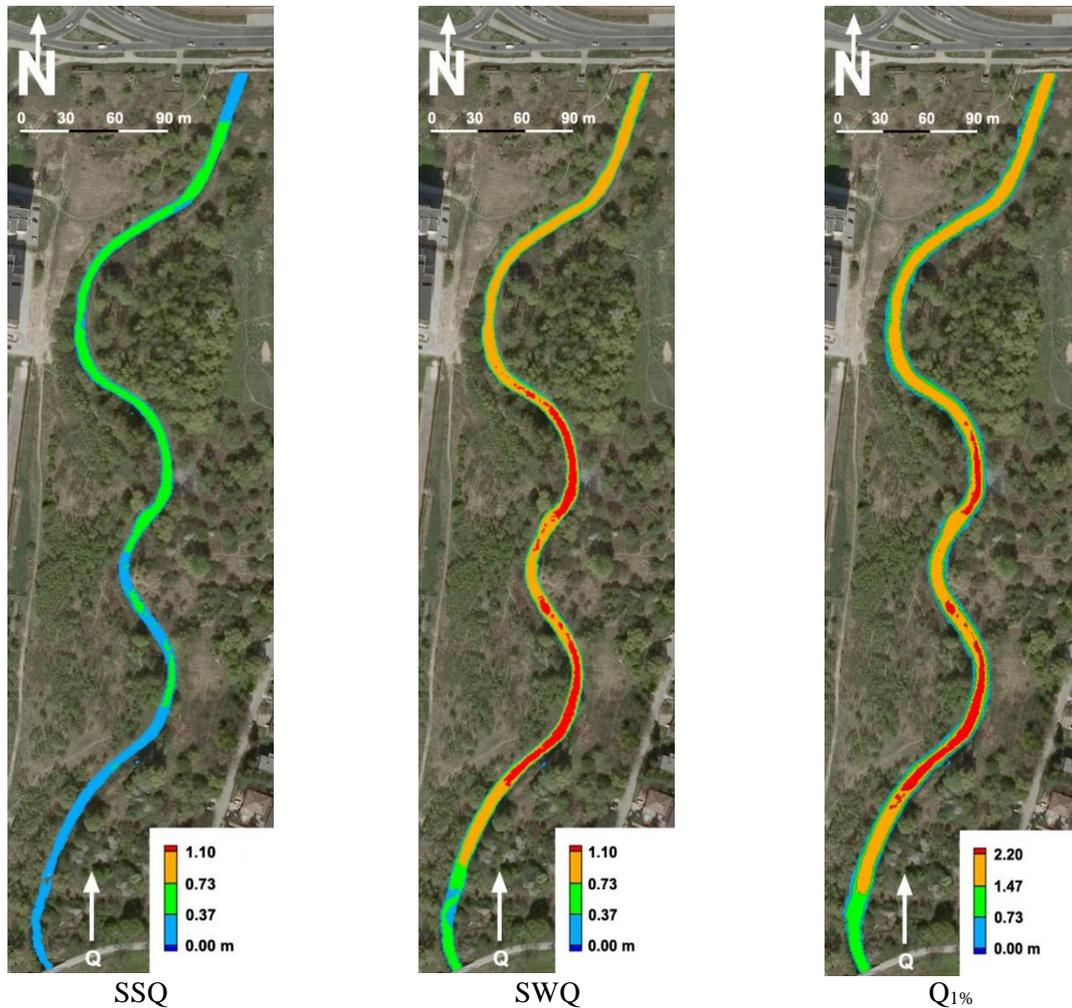
Fig. 3. The water depth in the watercourse for the multiannual mean low flow (a) and mean annual maximum flows (b)
