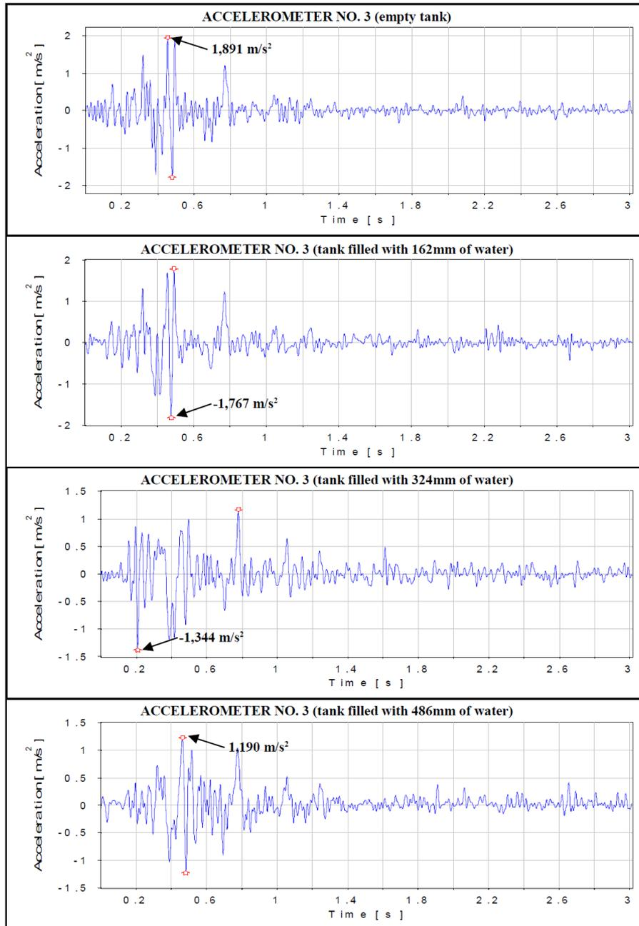
Fig. 6. Acceleration time histories under the Polkowice 2002 mining tremor (accelerometer no. 3)
