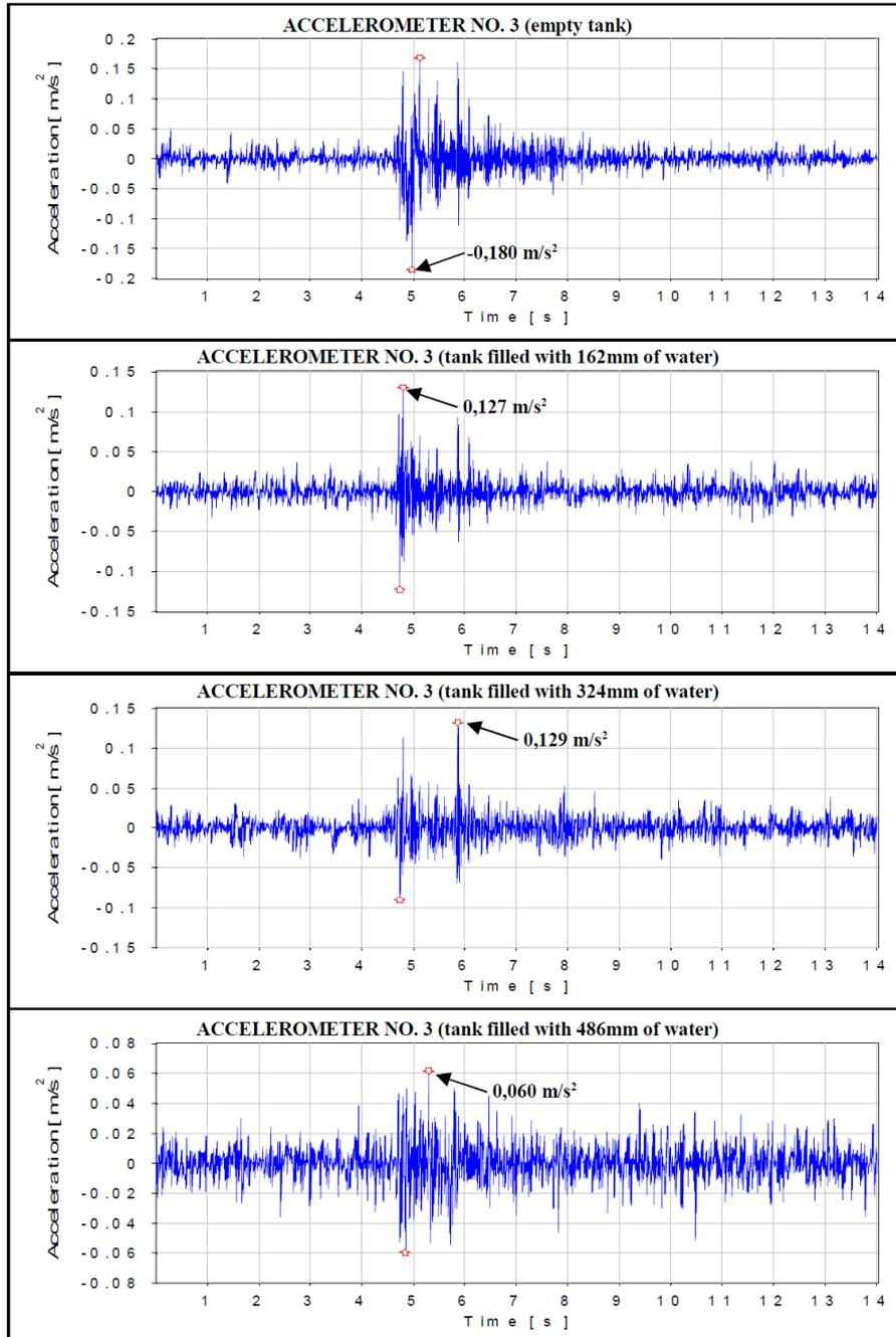
Fig. 4. Acceleration time histories under the Suwaki earthquake (accelerometer no. 3)
