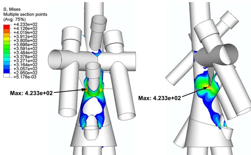
Fig. 5. Map of equivalent stresses in two different views in MPa – nonlinear analysis
