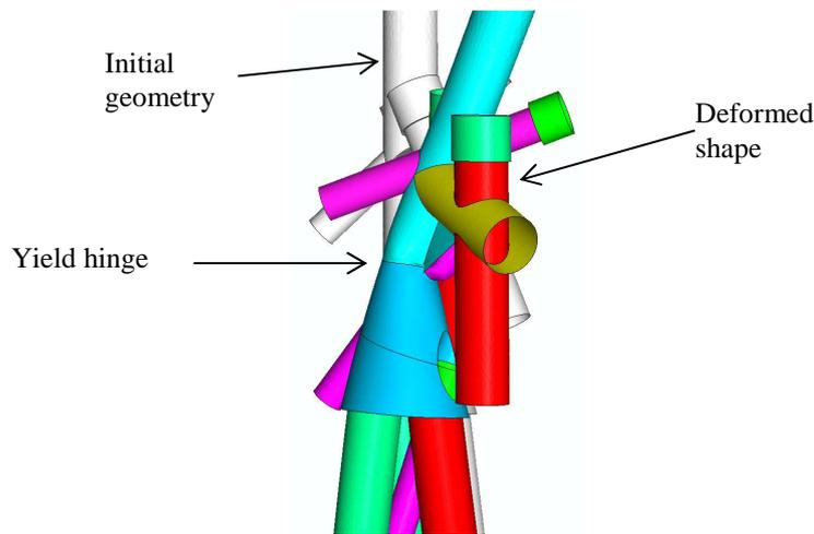
Fig. 6. The failure mechanism, scale 10:1
