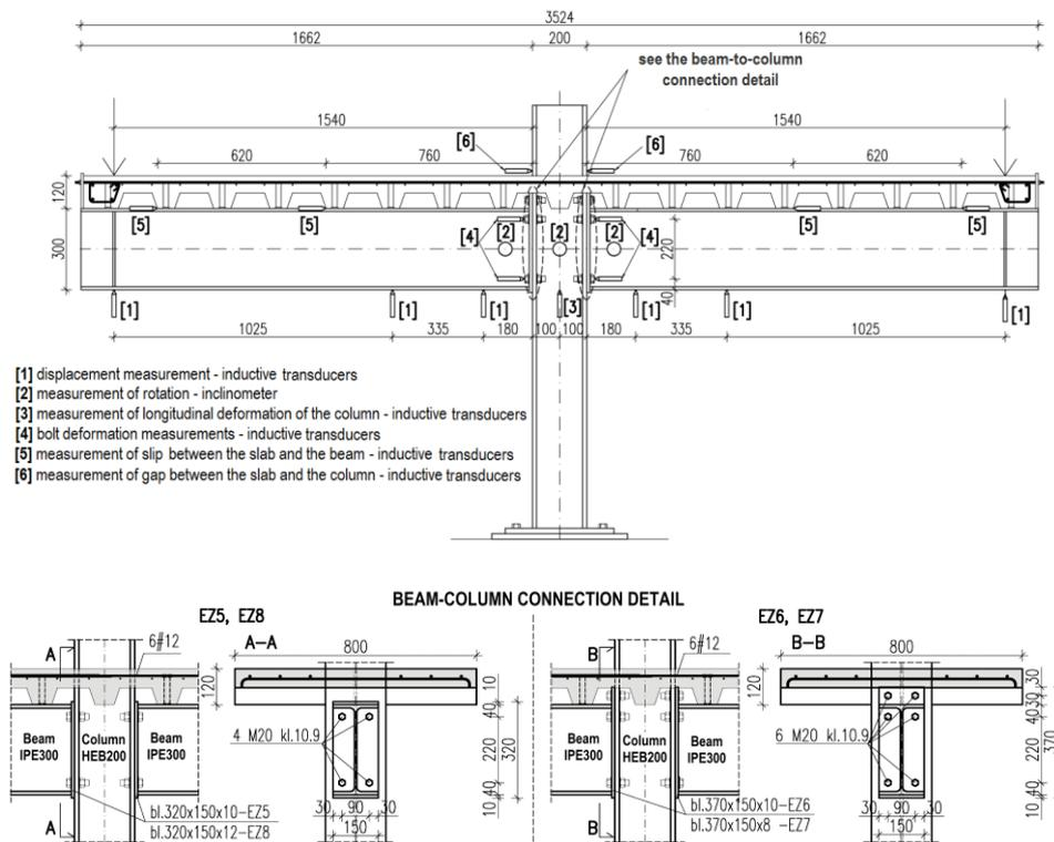
Fig. 2. Scheme of the tested elements
