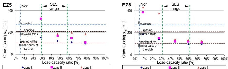
Fig. 7. The average crack spacing - specimens with the flush end-plate connections
