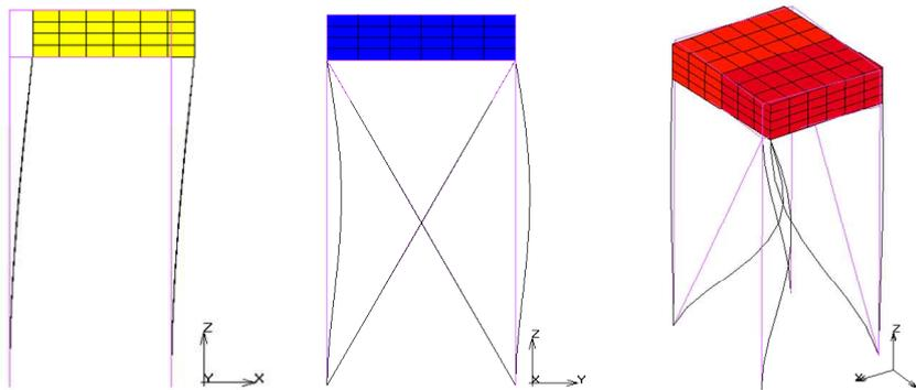
Fig. 4. Free vibration modes for Tower 1 and 3
