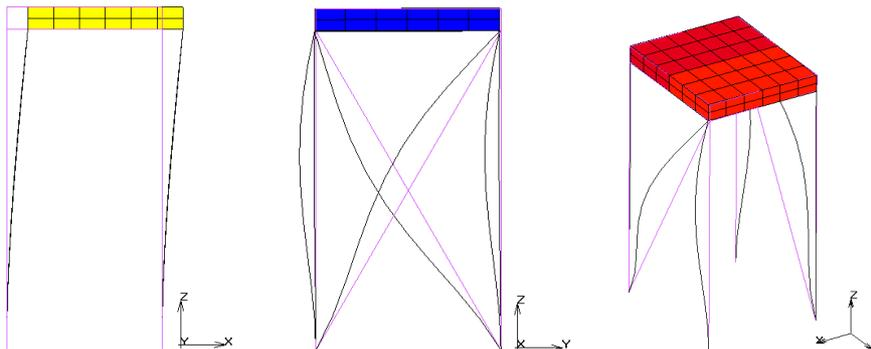
Fig. 5. Free vibration modes for Tower 2
