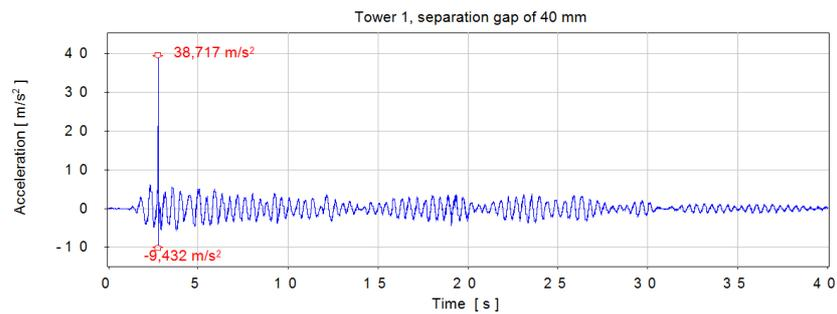
Fig. 2. Acceleration time histories for Tower 1 under the El Centro earthquake: a) Separation gap of 30 mm; b) Separation gap of 40 mm
