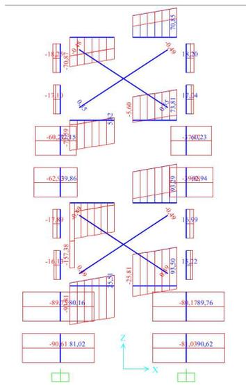
Fig. 5. Envelope diagram of shear forces, *kN*
