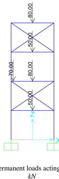
Fig. 3. Permanent loads acting on frame,  $kN$
