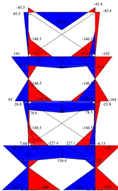
Fig. 9. Envelope diagram of shear forces,  $kN$
