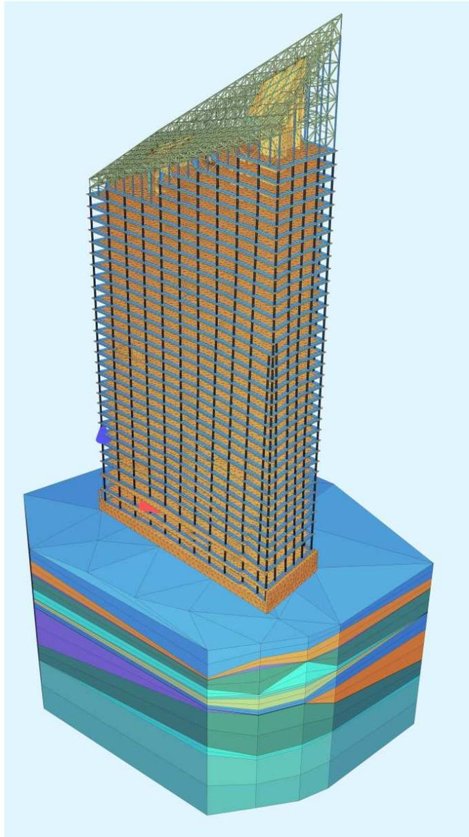
Fig. 1. FEA model of high-rise building in Minsk
