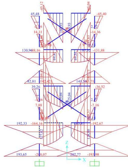
Fig. 8. Envelope elastic moments diagram (increased by the safety factor),  $kN \cdot m$
