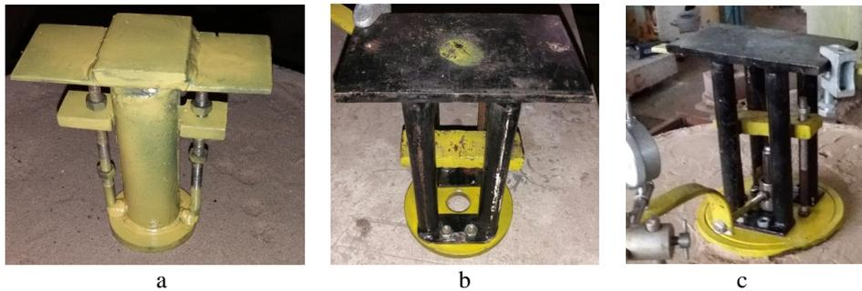
Fig. 3. The photo of plate model segments depending on pile diameter ( $d$ ) and conditional distance between piles: a –  $3d$ , (75 mm); b –  $5d$ , (125 mm); c –  $7d$  (175 mm)
