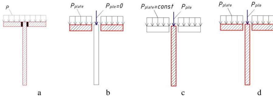
Fig. 4. Layout of load combinations of pile foundation elements: a – 1<sup>st</sup> test; b – 1<sup>st</sup> stage of II<sup>nd</sup> and III<sup>rd</sup> tests; c – 2<sup>nd</sup> stage of III<sup>rd</sup> test; d – 2<sup>nd</sup> stage of II<sup>nd</sup> test and 3<sup>rd</sup> stage of III<sup>rd</sup> test
