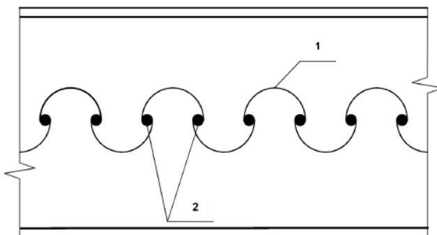
Fig. 4. Shape of web cut: 1 - cutting line, 2 - waste
