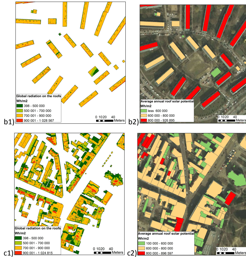
Fig. 6. Global radiation on building roofs (1) and solar potential of roofs (2) in \text{Wh/m}^2 in Bydgoszcz: a) a single-family housing estate; b) multi-family housing estate; c) city centre
