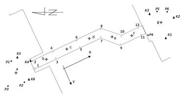
Fig. 1. Network point layout (P1 $\div$ P6 – reference points,  $1\div$ 12 – controlled points,  $a\div g$  – laser station points, K1 $\div$ K6 – adjustment points)
