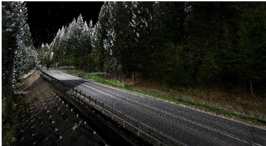
Fig. 4. Terrestrial laser scan within the analysed landslide
