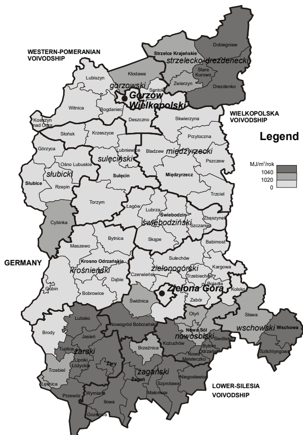
Fig. 12. The potential of solar energy that can be obtained with a solar collector [MJ/m 2 /year] (Source: prepared by the author, based on [18])
