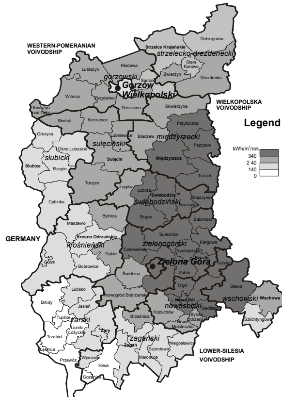
Fig. 8. The wind energy potential 60 m above ground level in [kWh/m 2 /year] (Source: prepared by the author, based on [18])
