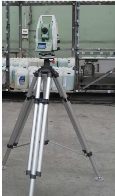
Photo 2. Coordinate laser station of the Leica brand, model TDRA 6000
