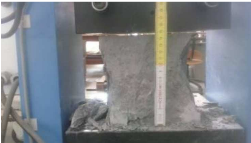
Fig. 4. Reading the soaking level at the turn of the sample
