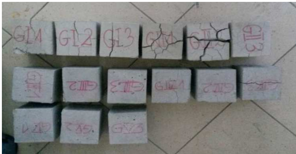
Fig. 5. Samples after frost resistance test (25 cycles)
