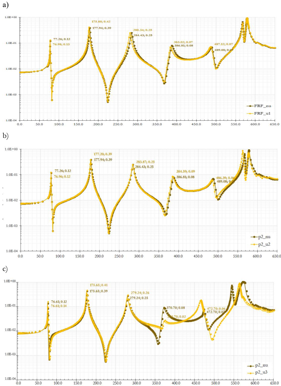
Fig. 10. Changes in resistance of models: a) U1, b) U2, c) U3.
