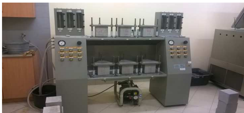
Fig. 6. Samples during the test of water-tightness
