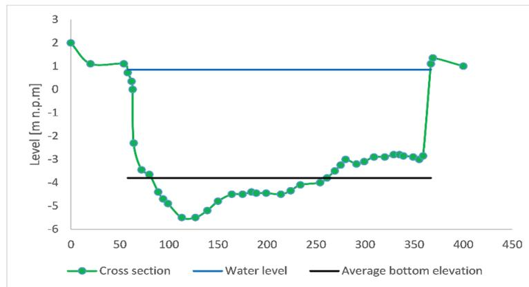
Fig. 3. Cross-section bathymetry
