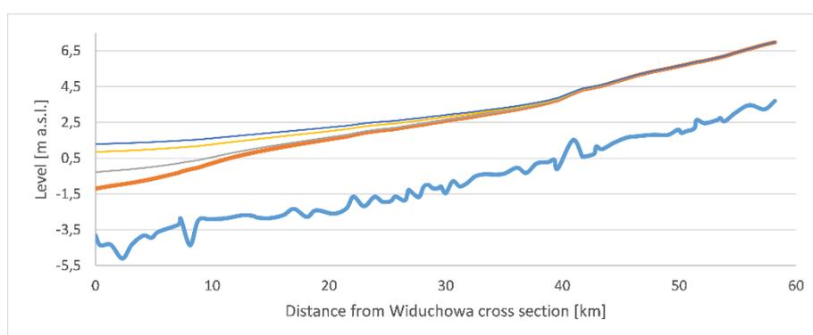
Fig. 4. Backwater curves for SSQ flows. Light blue – river bottom; orange – normal depth (without damming); grey - curve for  $Q = 599 \text{ m}^3/\text{s}$  and  $W = -0.275 \text{ m. a.s.l.}$ ; gold - curve for  $Q = 599 \text{ m}^3/\text{s}$  and  $W = 0.855 \text{ m. a.s.l.}$ ; blue - curve for  $Q = 599 \text{ m}^3/\text{s}$  and  $W = 1.292 \text{ m. a.s.l.}$
