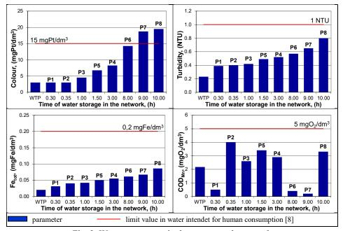
Fig. 3. Water parameters in the water supply network
