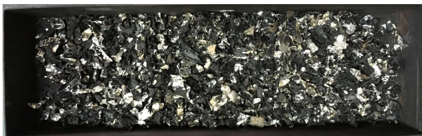
Fig. 9. The material after pyrolysis (PTp5)
