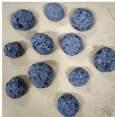
Fig. 1. Photo of manufactured electrically conductive aggregate
