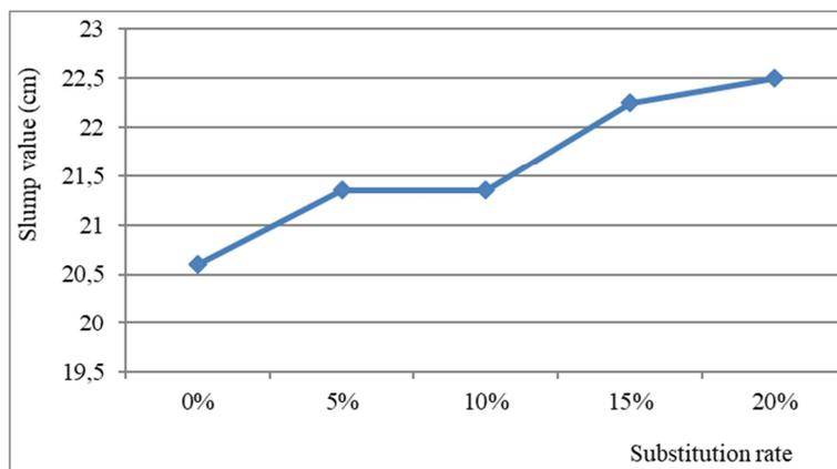
Fig. 2. Variation of workability as a function of substitution rate
