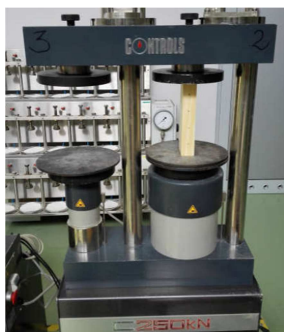
Photograph 3. Testing of wooden samples on the hydraulic press
