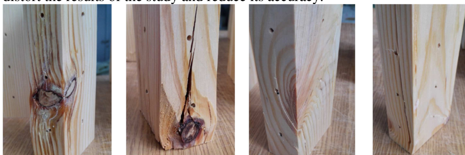
Photographs 5, 6, 7, 8. Samples rejected due to wood defects
