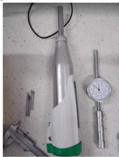
Photograph 1. Wood test sclerometer
