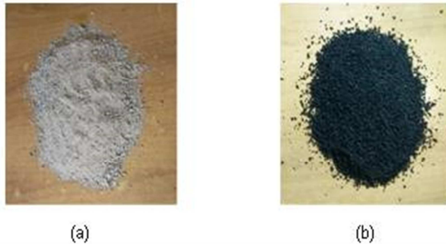
Fig. 1. a) Natural aggregates (sand), b) Rubber waste granulates (RW)
