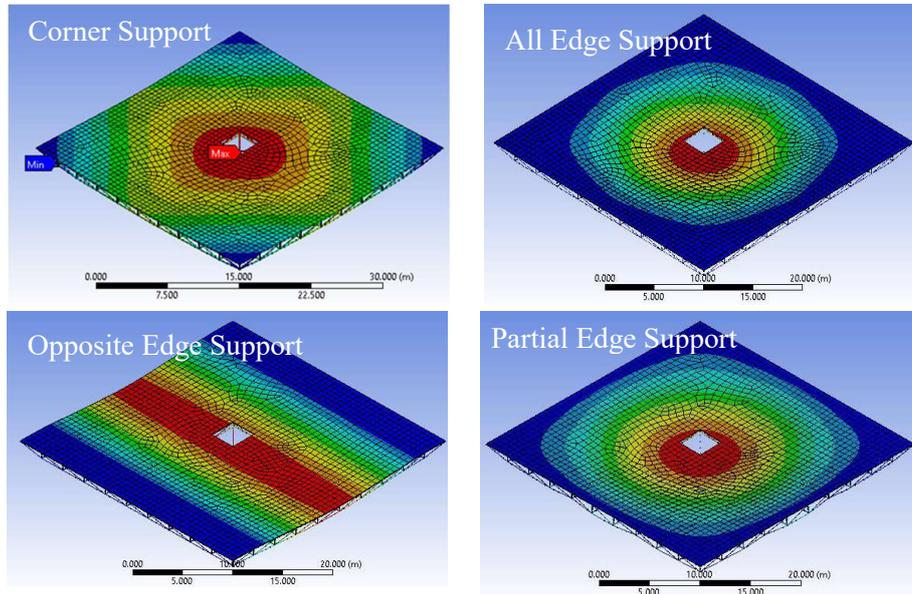
Fig. 8. Central maximum deflection of composite space truss - Opening 1
