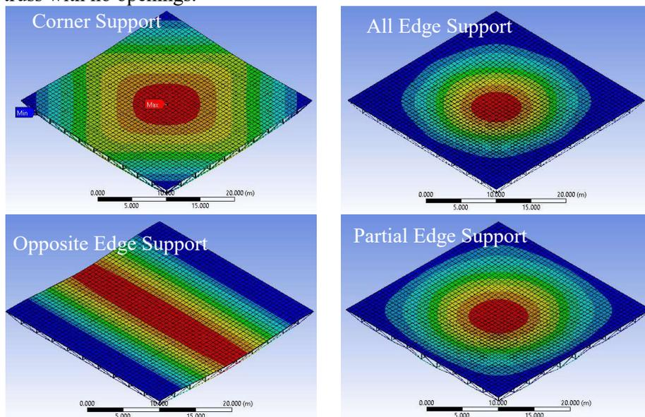
Fig. 7. Central maximum deflection of composite space truss - No Opening
