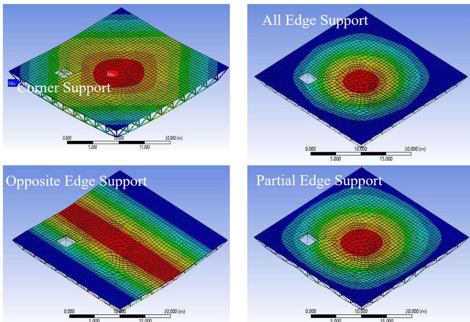
Fig.11. Central maximum deflection of composite space truss - Opening 4/13
