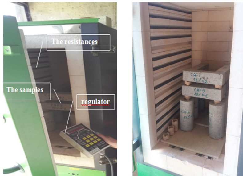
Fig. 6. Location of the concrete specimens in the furnace
