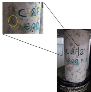
Fig. 17. The melting and ignition of AF fiber at 600°C temperatures
