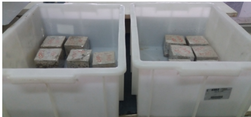
Fig. 8. Samples of dimensions 70x70x50 mm for the porosity accessible to water test and the capillary absorption test
