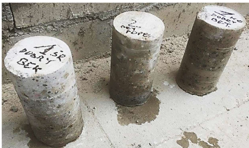
Fig. 19. Cores from the mid-span and support zones
