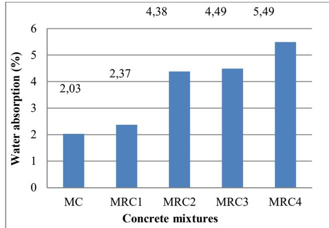
Fig. 11. Water absorption values of concrete mixtures
