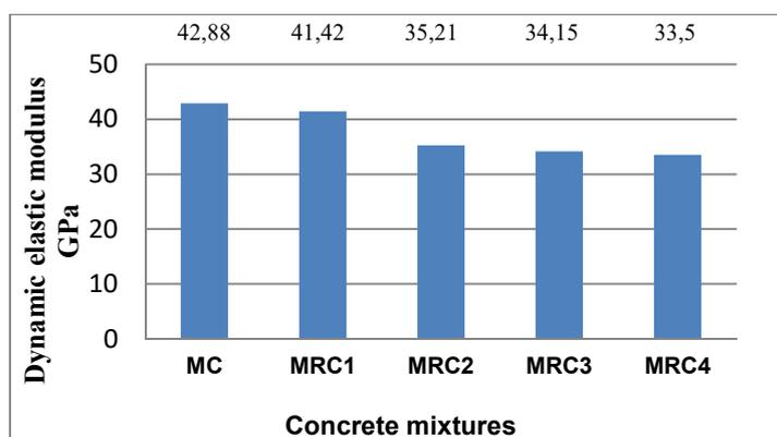
Fig. 14. Dynamic elastic modulus values of concrete mixtures
