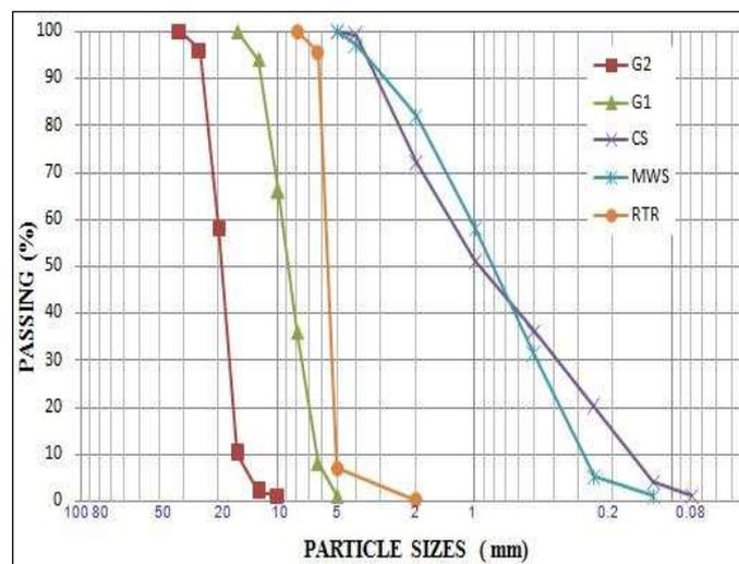
Fig. 2. Particles size distribution of aggregates
