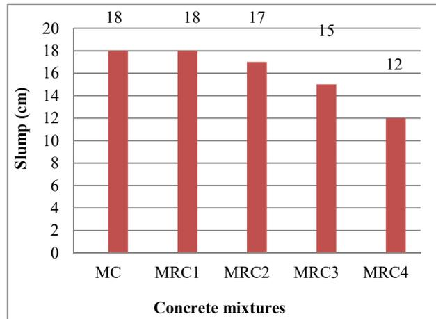
Fig. 3. Slump values of concrete mixtures
