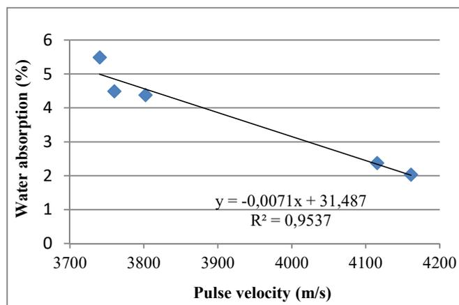
Fig. 12. Relationship between water absorption and pulse velocity
