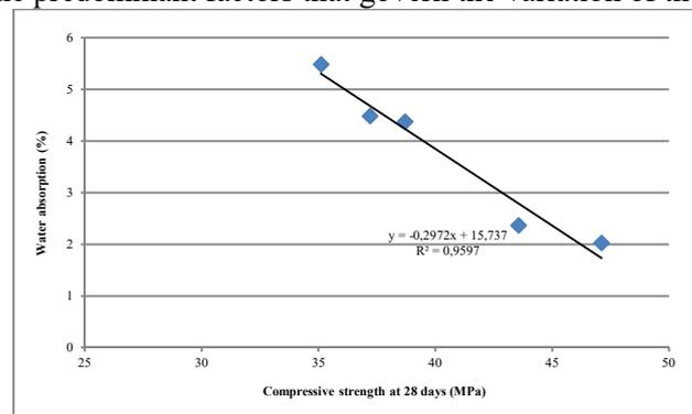
Fig. 13. Relationship between water absorption and compressive strength
