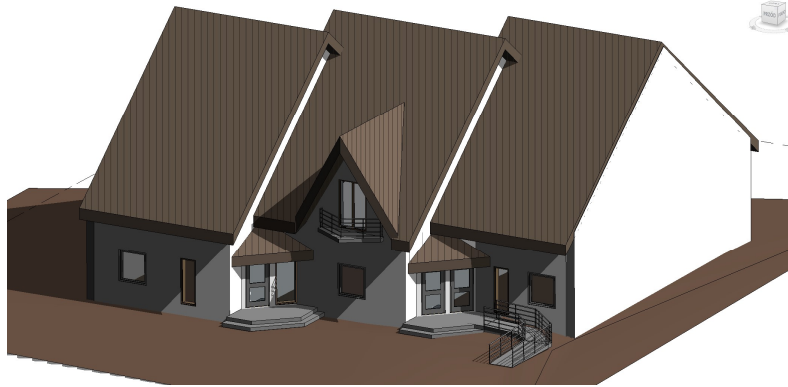
Fig. 11. Building model made in Autodesk Revit based on a dense point cloud
