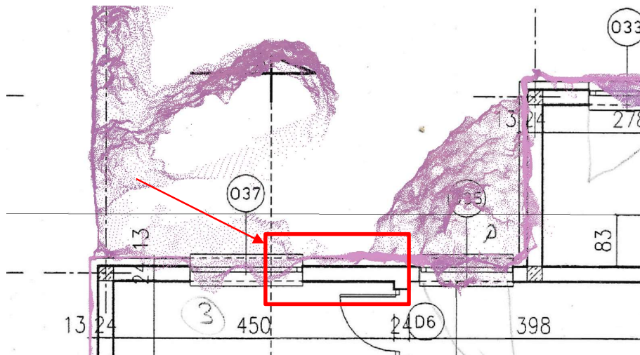
Fig. 10. Fragment of a point cloud with visible subdivision from drawing documentation
